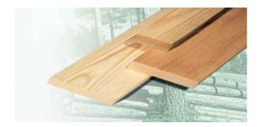
Length: 4 - 6 meters; Thickness: 22mm – 44 mm and more; Grade: I, II, III, IV; Species: spruce, pine; Mass of 1m<sup>3</sup>: 610-700 kg; Detail code FEACN: 4407109300 (pine), 4407109100 (spruce). The price for a 1m<sup>3</sup>coniferous cut board – 130-150 euro (depending on the grade and thickness)
